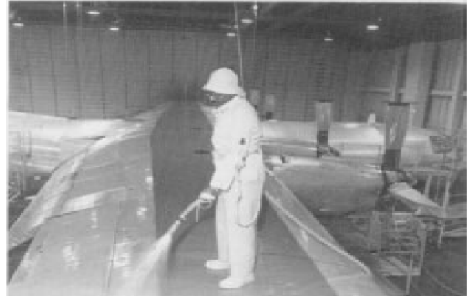
Wash rack workers need the protection of safety harnesses when working on the upper surfaces of the aircraft.
