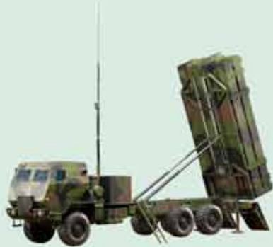
Launcher – Transportable, tactically mobile, rapid-reload design
