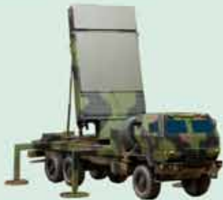
Sensors – UHF Surveillance Radar and X-band Multifunction Fire Control Radar both protect with 360-degree coverage
