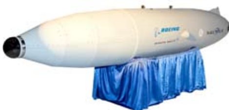
The IRST installation in the prototype fuel tank
