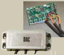
Data Acquisition Controller (DAC)
