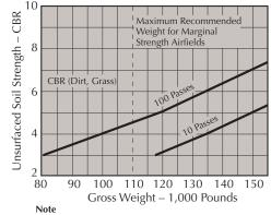
Number of Passes Is Based on Main Landing Gear Tire Inflation Pressure for Marginal Strength Airfields. A Pass Is Defined as One Landing and One Takeoff.
