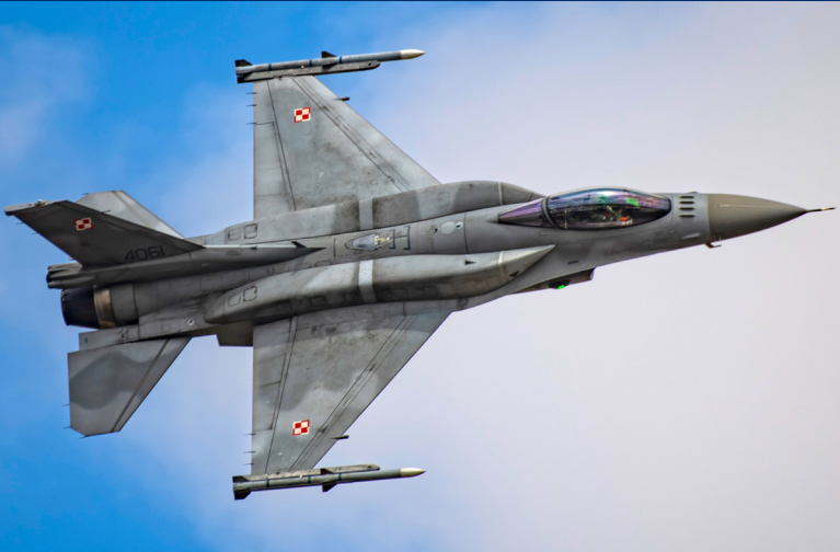
A Polish Air Force F-16C Block 52+ takes flight at RIAT 2025 with conformal fuel tanks, highlighting the jet's extended range and operational versatility.
