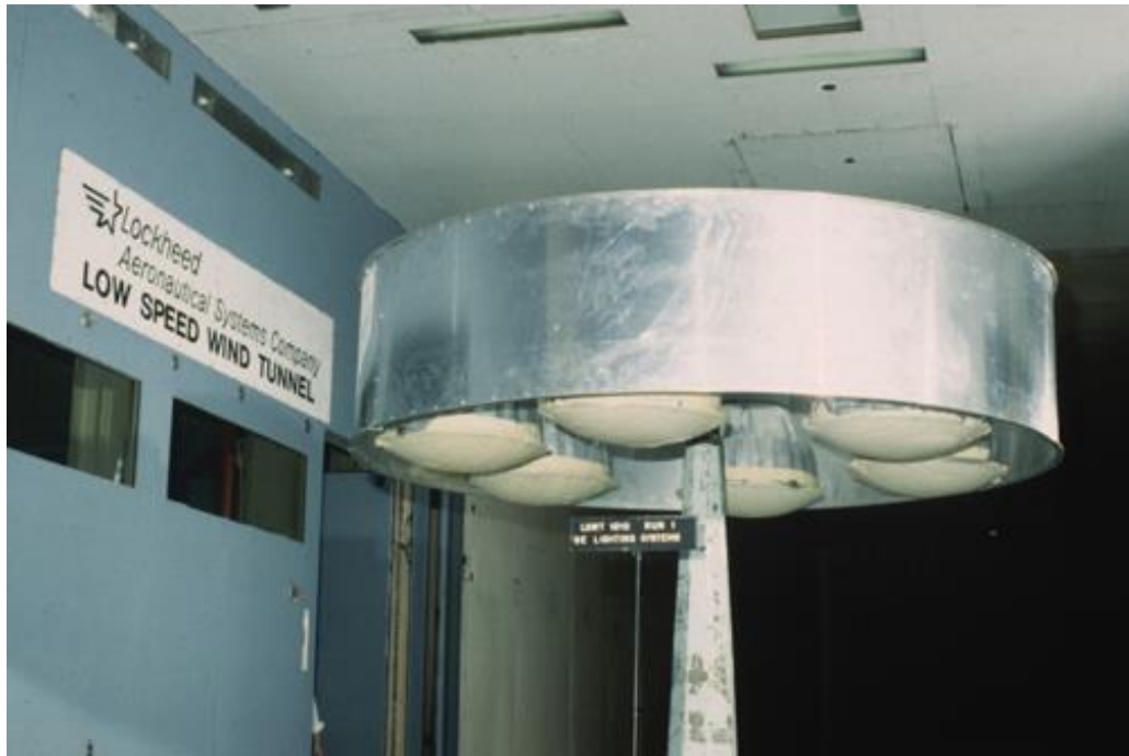
Figure 15. Architectural Model (Lighting Fixture) Installation.
