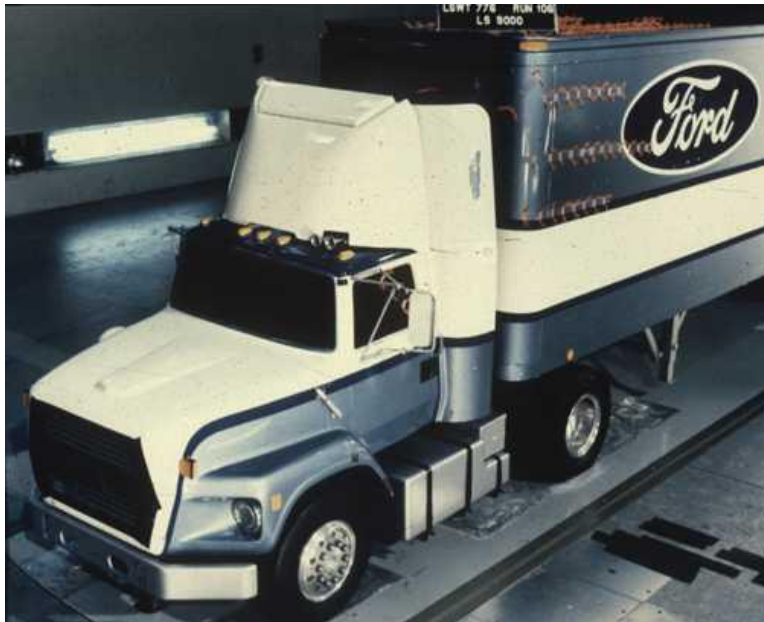
Figure 21. 0.3-Scale Tractor/Trailer Model Installation.
