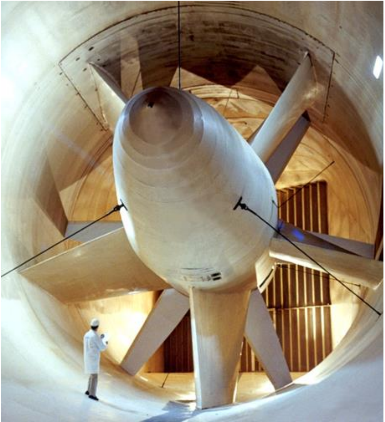
Figure 38. Main Drive System – View Looking Upstream.
