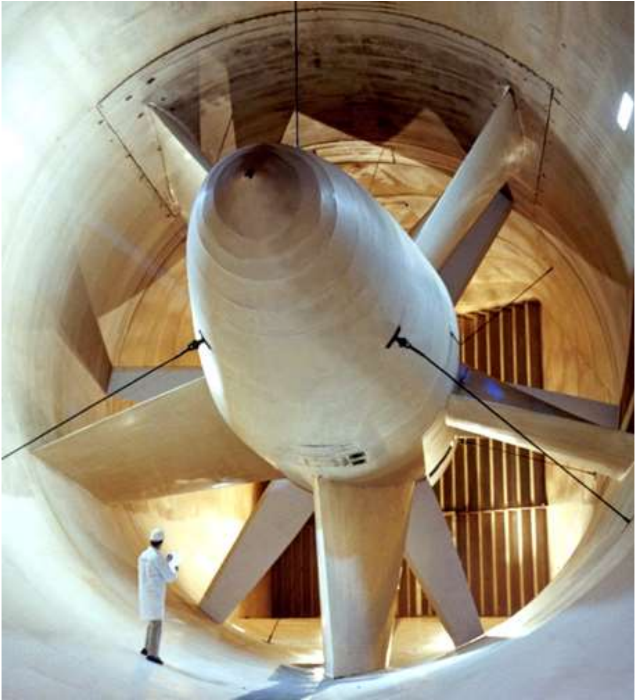
Figure 38. Main Drive System – View Looking Upstream.
