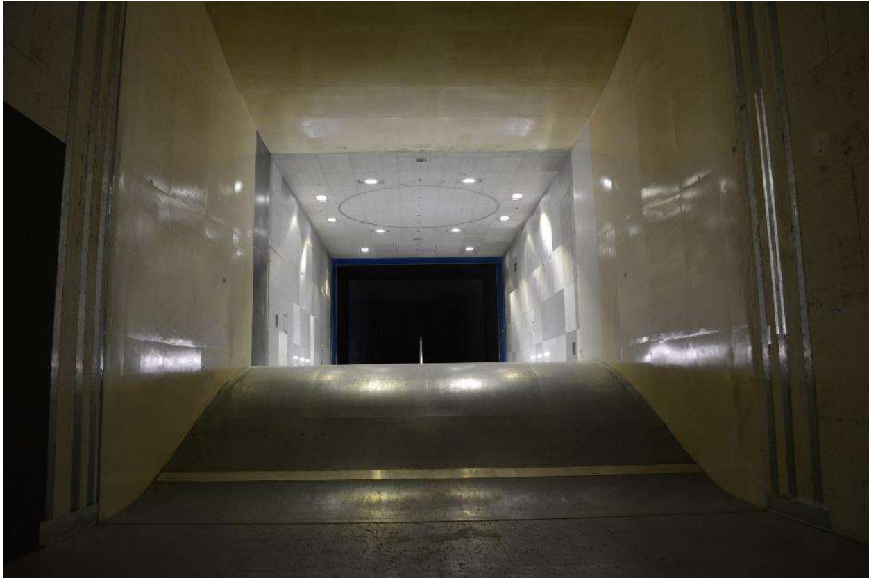
Figure 5. View Looking Downstream Through Both Test Sections.
