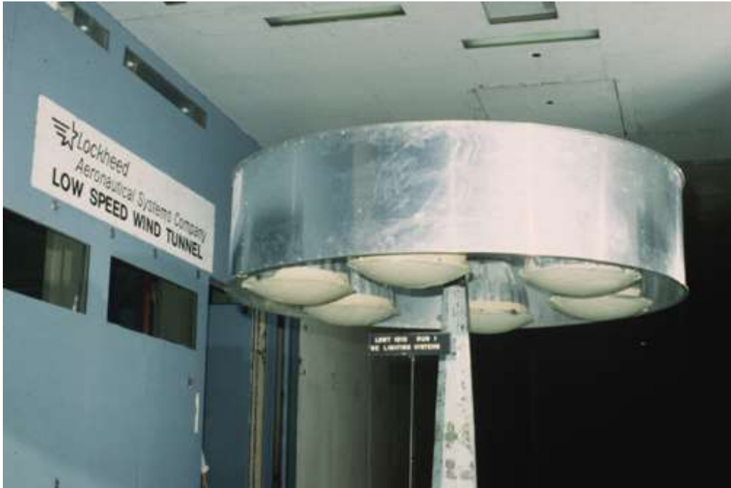
Figure 15. Architectural Model (Lighting Fixture) Installation.
