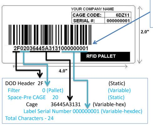
RFID Tag ID – Enter into TMS on THU Create Screen. Barcode can be used to populate field in TMS
