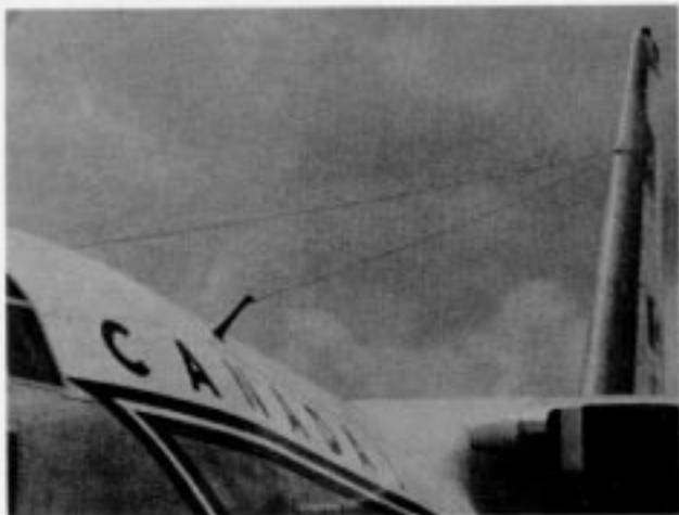
Figure 1. The forward end of each HF antenna wire is anchored to an AML-61 antenna mast.
