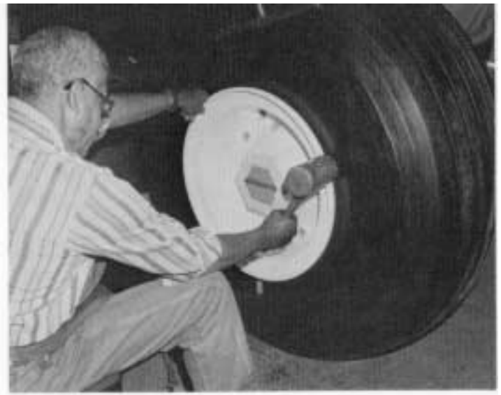
Putting wheel halves into tire.
