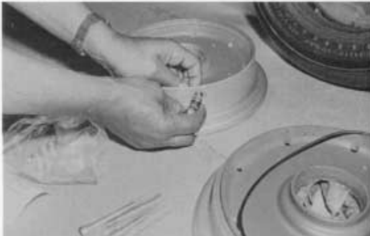
inserting valve stem into wheel.
