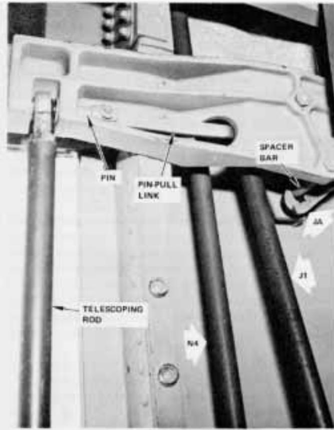
The second check is to see that the pin-pull link actually pulls the pin completely free of the rod. On the surface, this may not seem worth mentioning; however, on certain aircraft, unrelated modifications have caused the pin-pull link to bind and not actually pull the pin from the rod.
