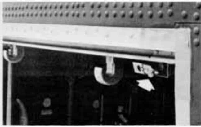
Figure 14. The door closed switch is located near the upper aft corner of the door opening.
