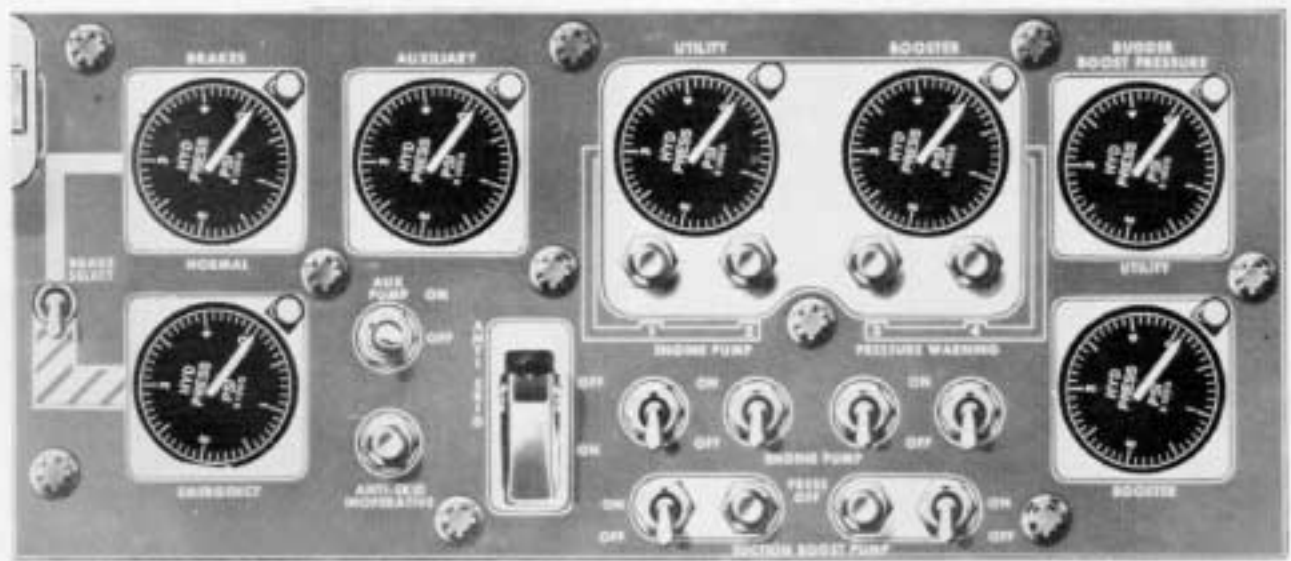
Hydraulic control panel – copilot's instrument panel.
