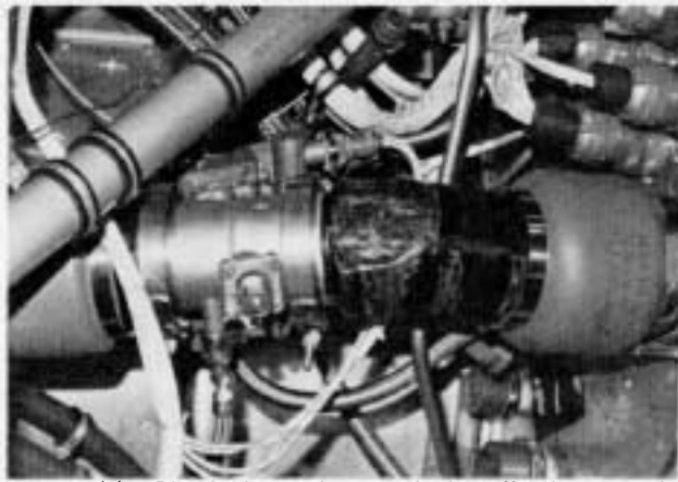
Above Left: Bleed air regulator and shutoff valve – engine nacelle. Right: Cargo compartment air conditioning unit – forward right wheel well fairing.
