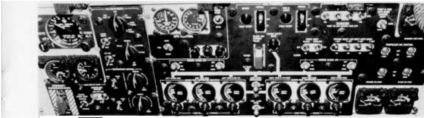
Anti-icing system control panel ~ flight station overhead control panel.
