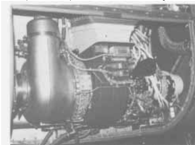
Auxiliary power unit—forward left wheel well fairing.
