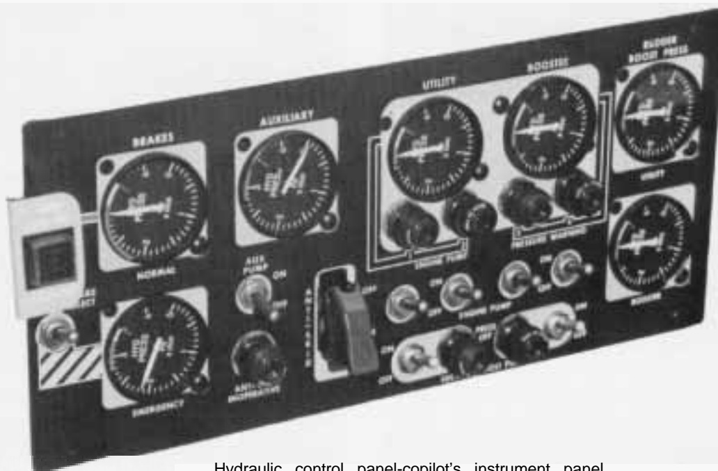
Hydraulic control panel-copilot's instrument panel.
