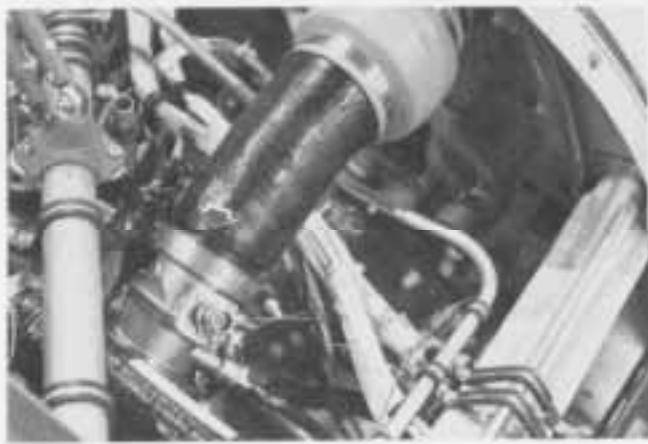
Bleed air regulator and shutoff valve-engine nacelle
