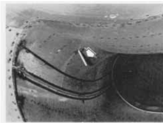
Engine air inlet ice detector.
