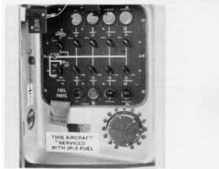
SPR panel and receptacle-aft right wheel well fairing.
