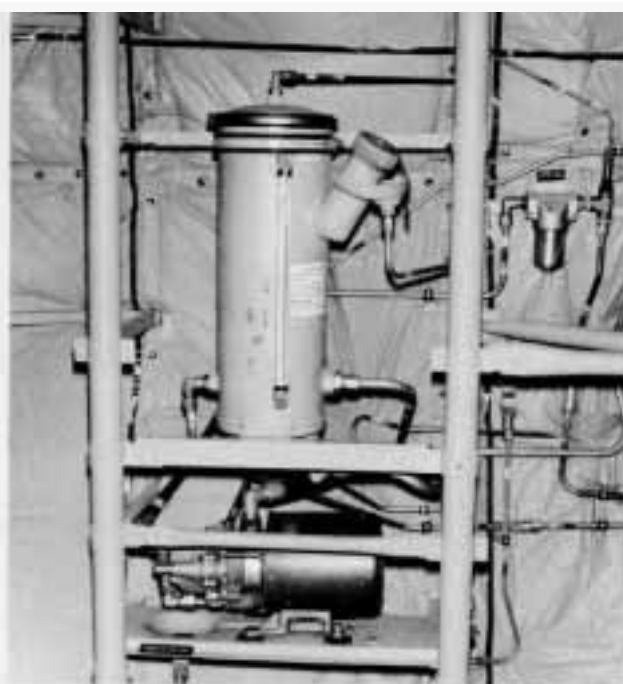
Drain the auxiliary system reservoir when removing system pump, ramp and door manifold, or hand pump.
