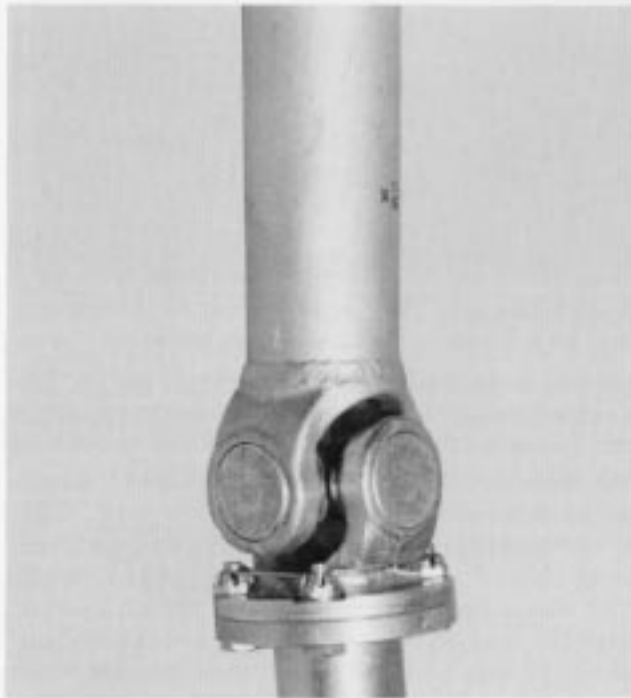
MLG torque shaft lower universal joint, typical of airplanes built prior to LAC 5162. Note the bolted coupling.
