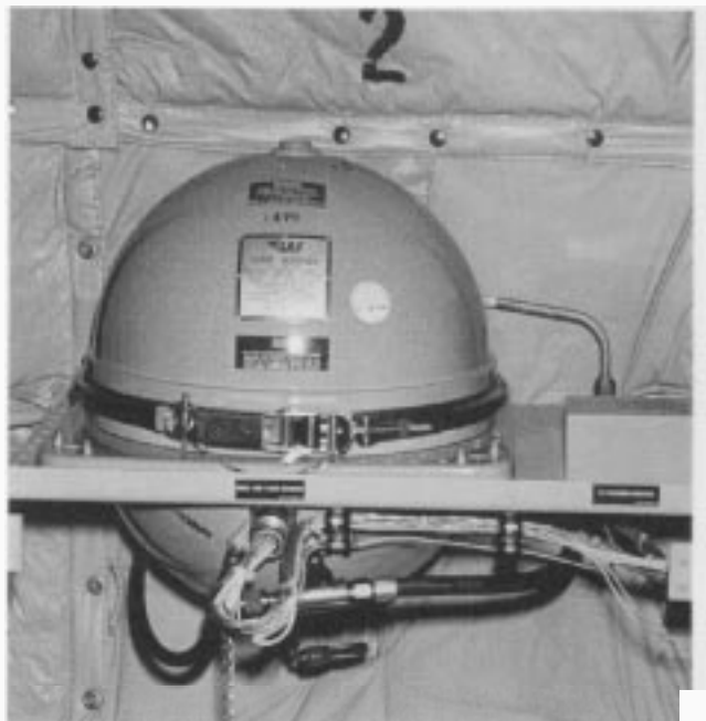
Figure 1 The 109-series FDR was mounted in a spherical, protective container.
