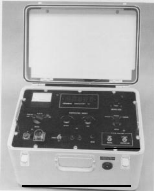
Figure 2 (above). For flight-line TD system checking, the portable PN 3402893-1 test set provides an excellent selection of on-aircraft functional tests.
