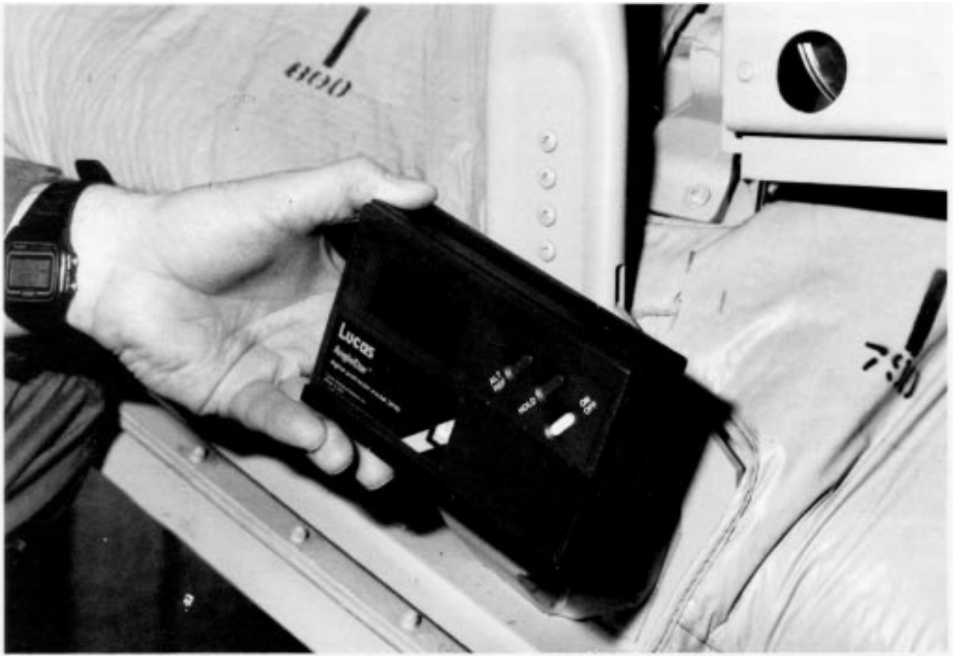
The heart of the new rams hook retainer identification tool is the digital protractor, a high-tech “hand” tool now in wide use in civil engineering and the construction industry.
