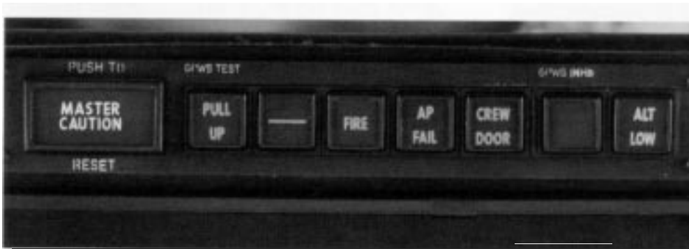
The MACAWS includes installation of a master caution light and a set of alert warning lights in the glareshield directly in front of each pilot.
