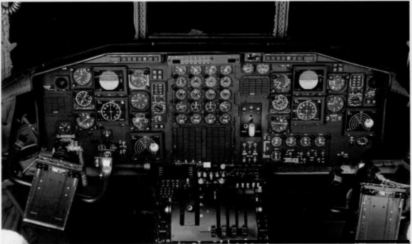
By day: the NVIS-compatible cockpit features a clean new layout, updated instrumentation.
