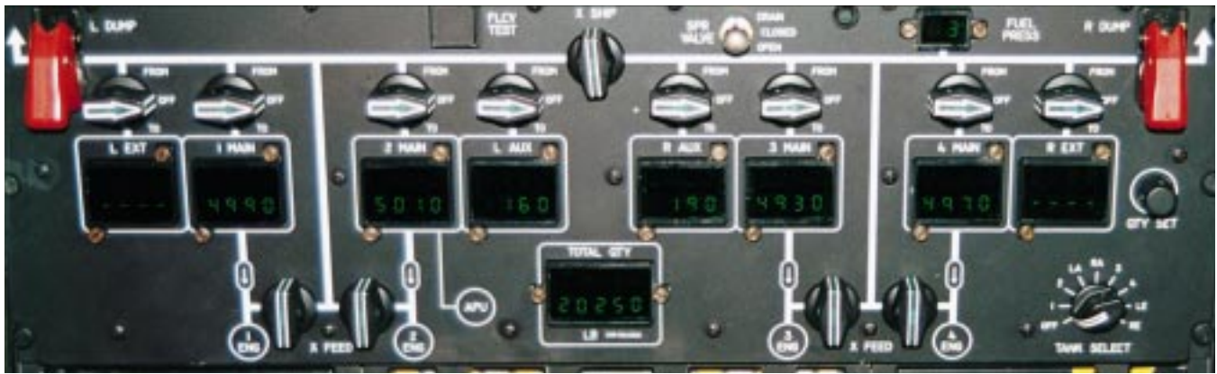
Figure 2. Fuel Control Panel located on the overhead console.
