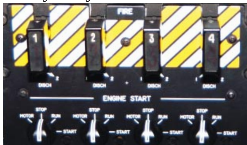
Figure 3. Engine Start and Fire Control Panel.
