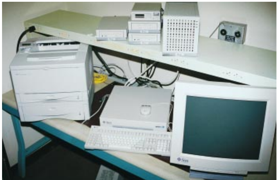
This is a typical GMS. Components shown include the monitor, keyboard, processor, CD drive, RMM interface, and other peripherals.
