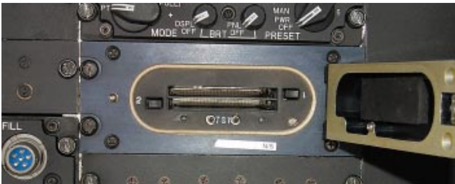
Right: The RMM loads directly into the DSDTS.
