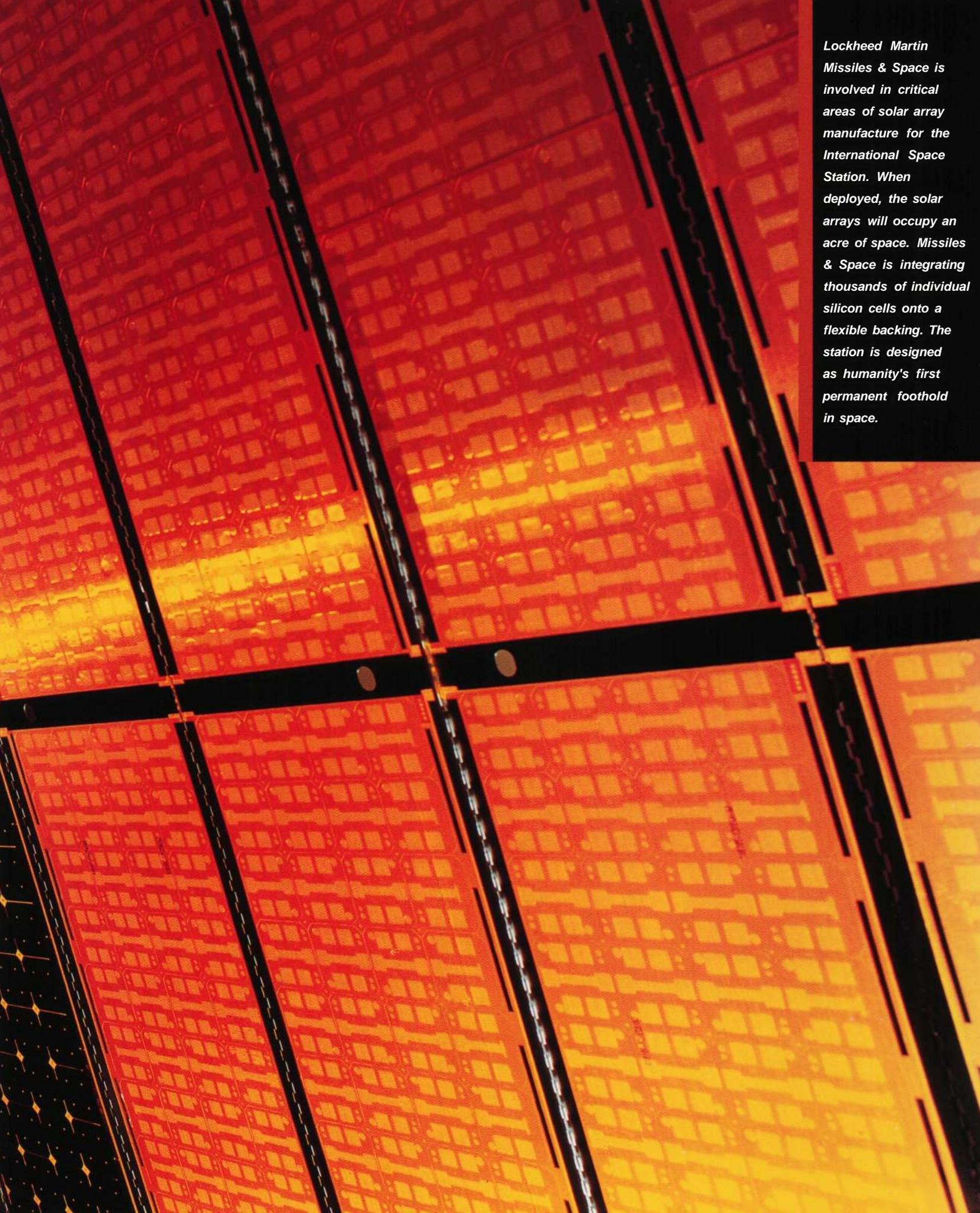
*Lockheed Martin Missiles & Space is involved in critical areas of solar array manufacture for the International Space Station. When deployed, the solar arrays will occupy an acre of space. Missiles & Space is integrating thousands of individual silicon cells onto a flexible backing. The station is designed as humanity's first permanent foothold in space.*
