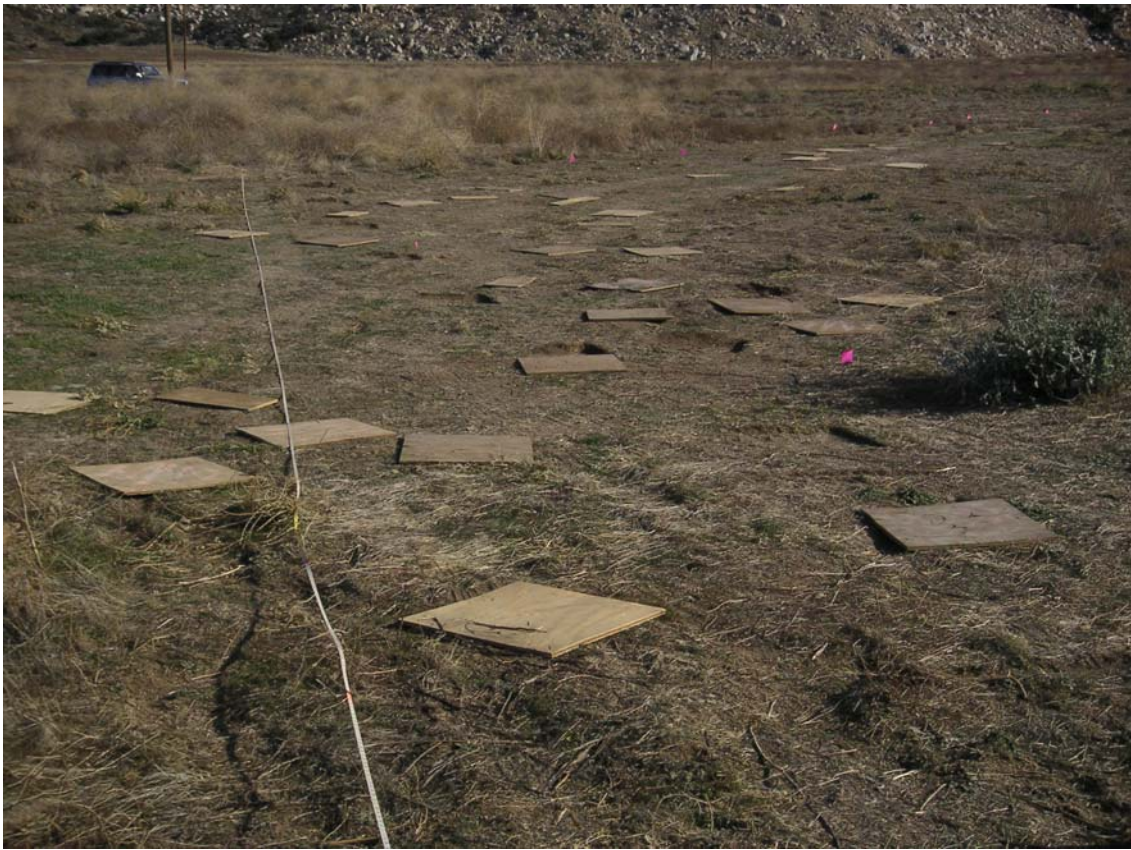
Seismic line location with SKR load spreading boards, Site 1 (Potrero Creek), 12/07/05
