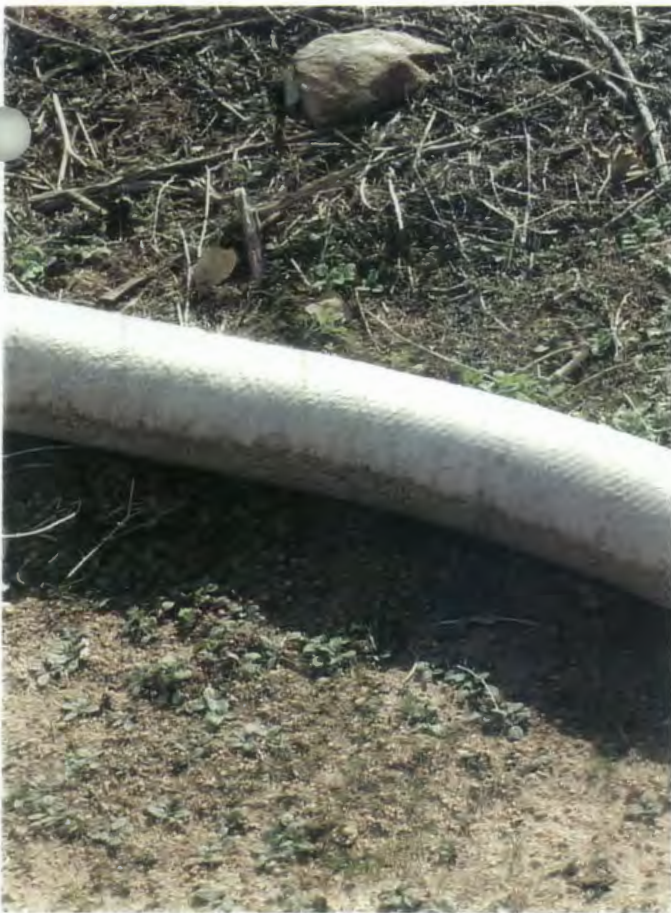
Site 1, Asbestos Transite Pipe Debris Scattered on Hillside Around Buidlings 308 and 305
