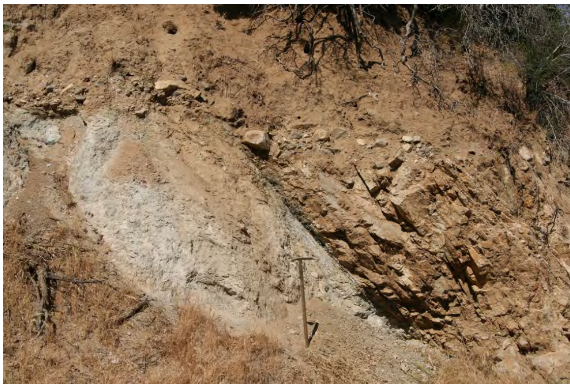
Photo 22. Goetz fault, dipping 50° north. The fault juxtaposes metamorphic rocks on the left with biotite-hornblende tonalite on the right. Fault zone is about 10 feet thick. Fault is overlain by conglomeratic stream deposit and colluvial material. Note offset basal bed with offset down to the right.
