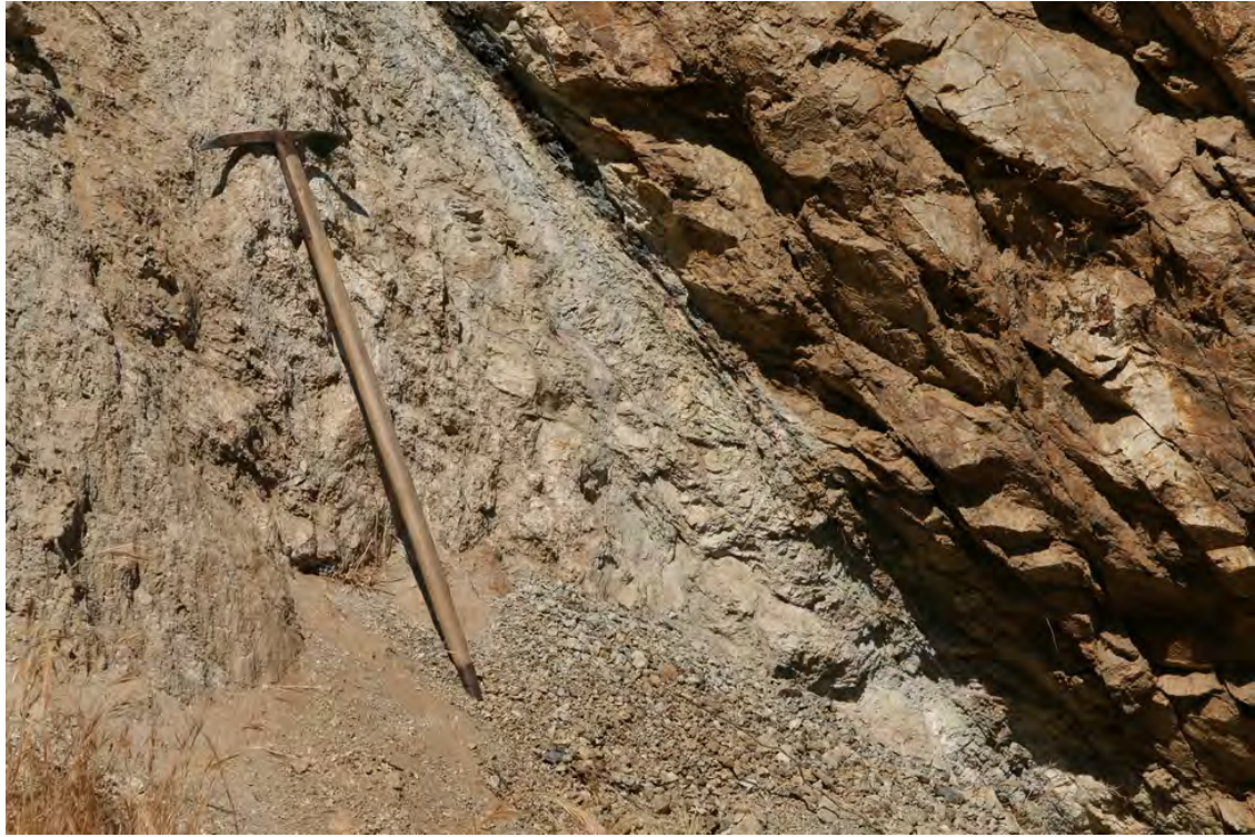
Photo 23. Close up of the Goetz fault showing 1-3-inch-thick dark-colored gouge.
