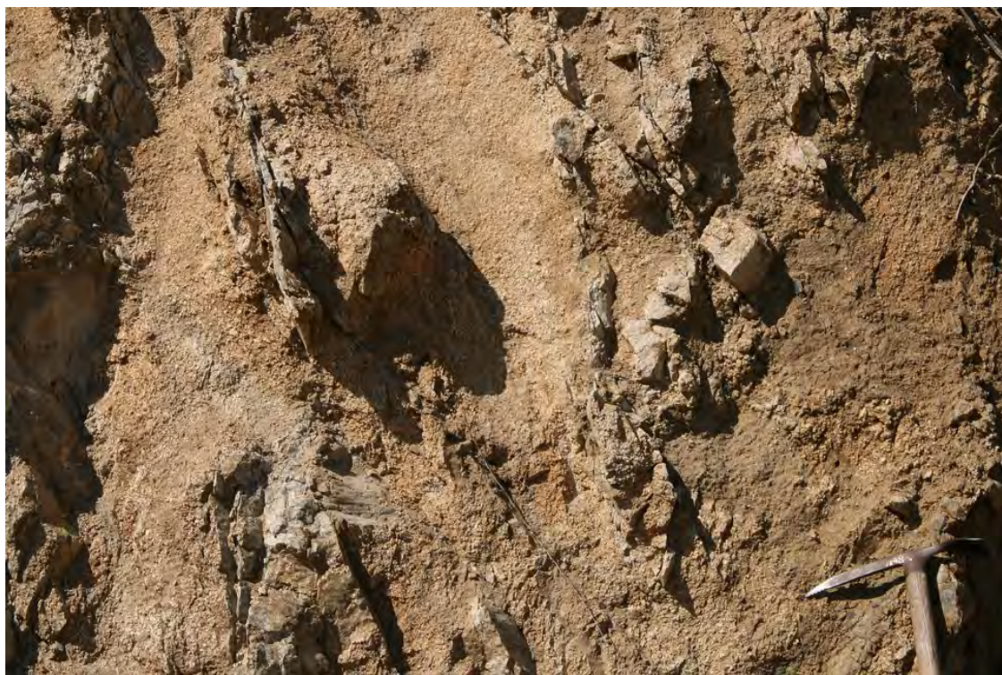
Photo 25. Detail of the shear zone. Note some slickensides oriented near normal to the outcrop face and other shears oriented parallel to the outcrop face with horizontal slickensides.
