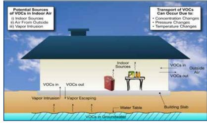
Indoor air quality may be affected if the contaminated vapor travels through cracks or openings in the foundation and enters the building. Vapor intrusion can occur in any type of building — regardless of age or construction — through a crack or opening in a basement, crawl space or foundation slab.
