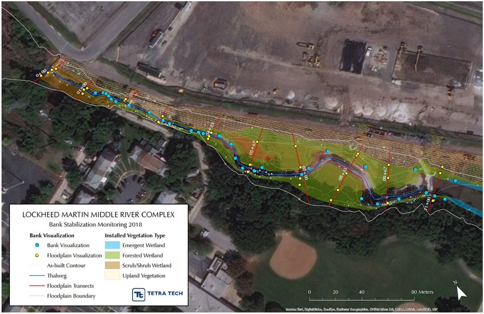
Figure 4-11. Map of Cow Pen Creek study area showing 2018 streambank and floodplain field survey points, along with as-built survey topography. Floodplain transect start points (yellow points closest to stream along transect) were field-placed at top of bank on both sides of stream. As-built survey is from December 2017; Upland and wetland vegetation types are from the November 2017 revegetation plan (Tetra Tech 2017).
