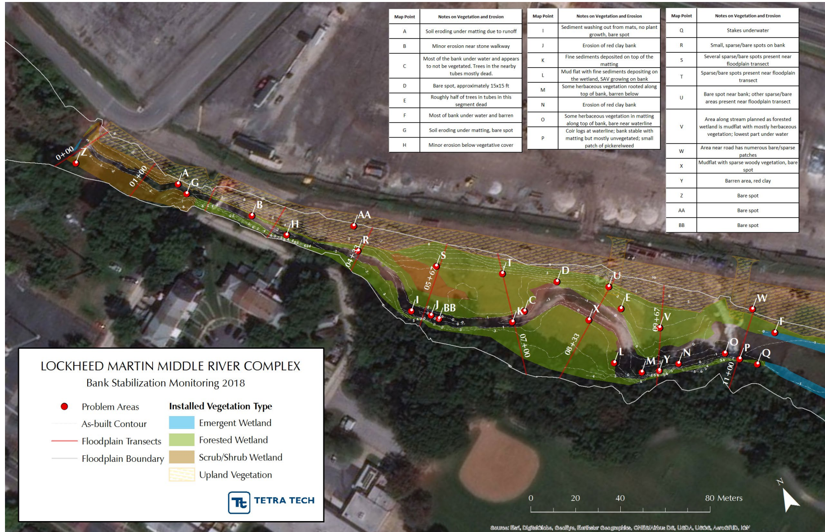
Figure 4-9. Map of Cow Pen Creek study area showing 2018 locations of areas noted based on concerns for erosion or vegetative cover condition. Upland and wetland vegetation types are from the November 2017 revegetation plan (Tetra Tech 2017).
