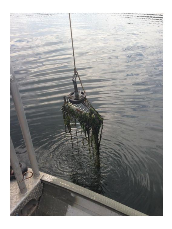
Figure 2. Modified rake used for conducting SAV surveys.
