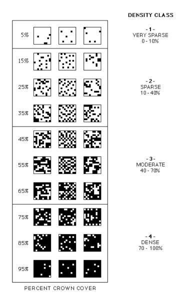
Figure 3. Scale used to measure the density of SAV rake survey grabs. The scale is based on a modified Braun-Blanquet (1932) scale with values ranging from 0 (no plants present) to 4 (70-100% cover).
