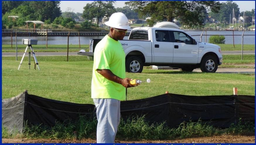
Air monitoring is performed using a portable device, called a Photoionization Detector (PID), to measure levels of volatile organic compounds in the air to protect site workers, employees and neighbors.
