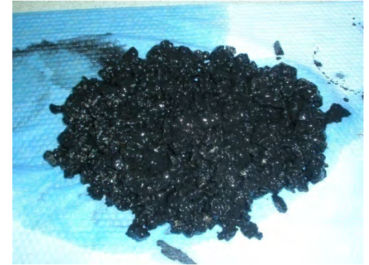
Above: Intact AG+PAC 5% after perm test
