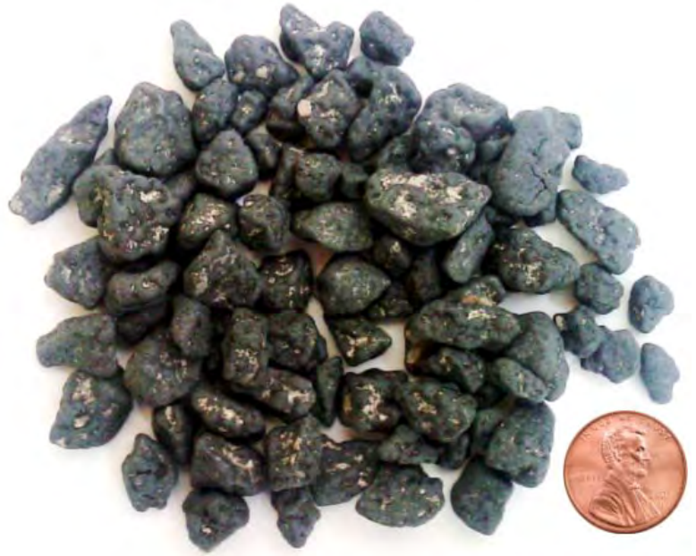
Figure 1. Configuration of PAC-coated particle.
