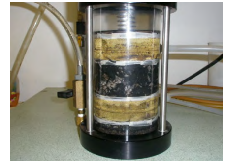
Above: Flex-wall permeameter – Flow 14,774 cm/day or greater used in three runs - Significantly in excess of a conservative 5 cm/day without material loss through sand pack
