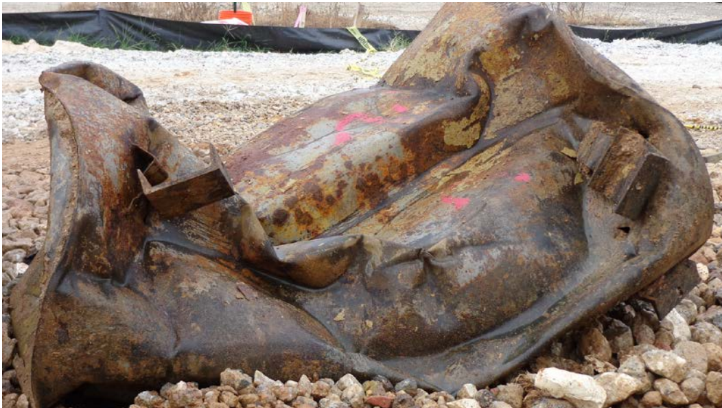
Close-up of UST #2 following extraction and washing
