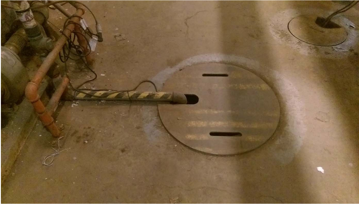
Photo 4 – Large cover plate (CP) with 92.11 ppb detection of trichloroethene using the Frog 4000™ .
