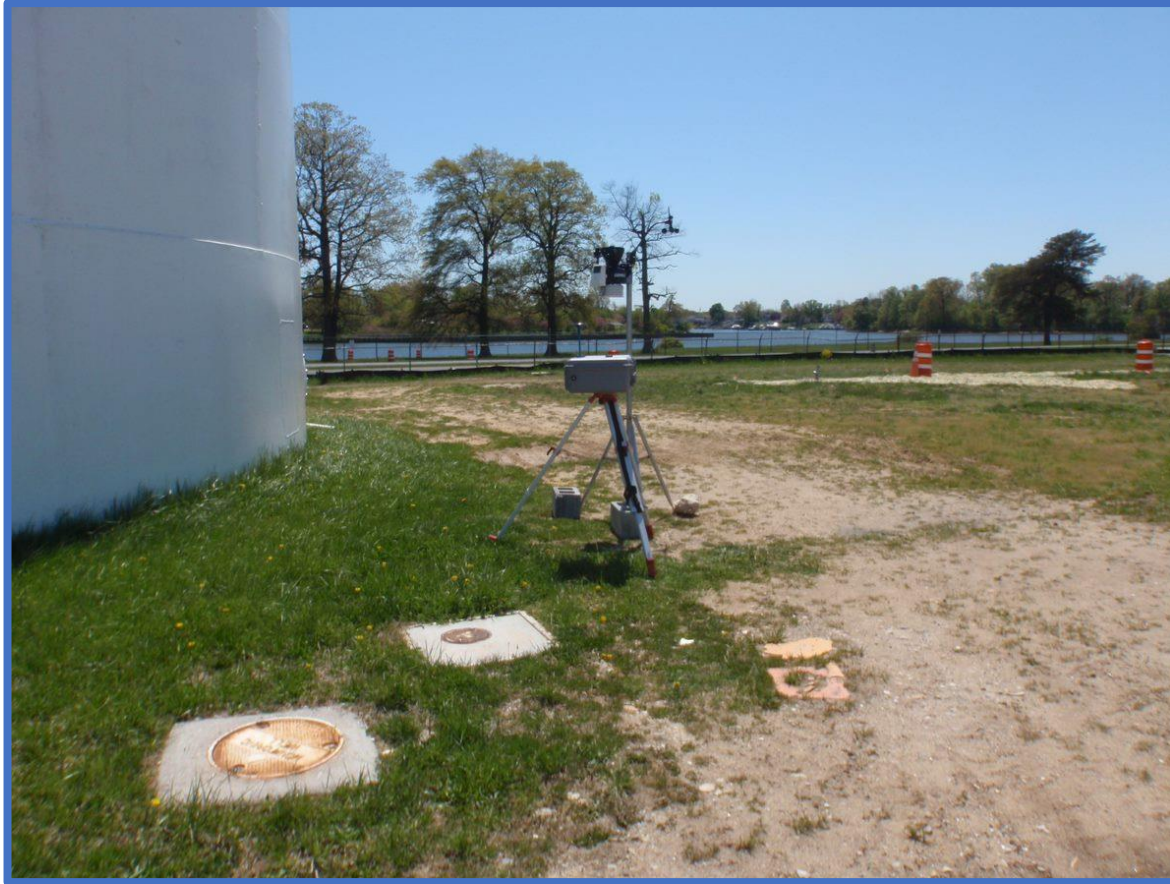
Air monitoring at the perimeter of work ensures dust from the site is managed.
