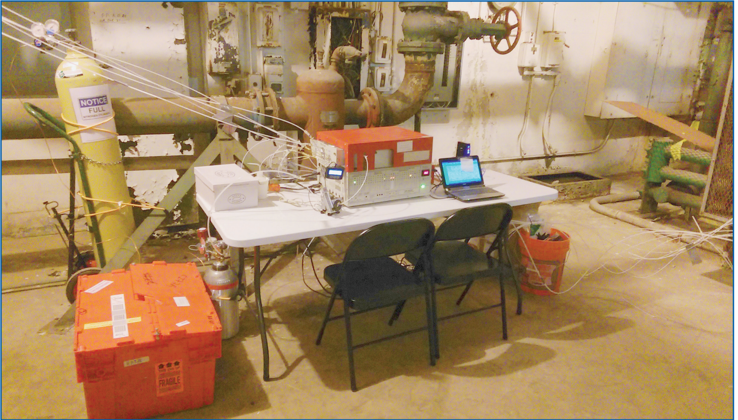
Sampling equipment was more complex than in previous sampling activities, and included extending tubing throughout the southern end of the basement and into the middle of the basement, and into subfloor drainage structures
