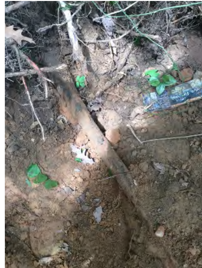
1.5" steel pipe located approx 1.5' bgs.
