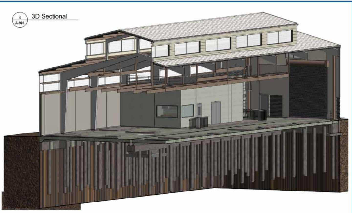
A rendering of the groundwater treatment building shows the concrete foundation piles. The piles extend through the former dump to the underlying natural sand formation to provide a strong foundation.
