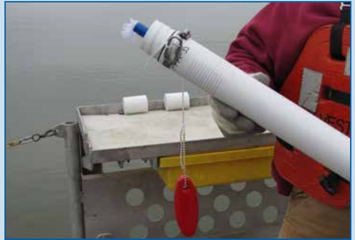
View of water flow sensor, also called Passive Flux Meter
