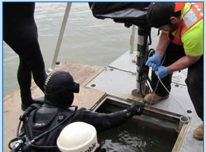
Divers installed and retrieved water flow sensors
