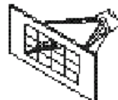
Special Purpose Intake Screen
