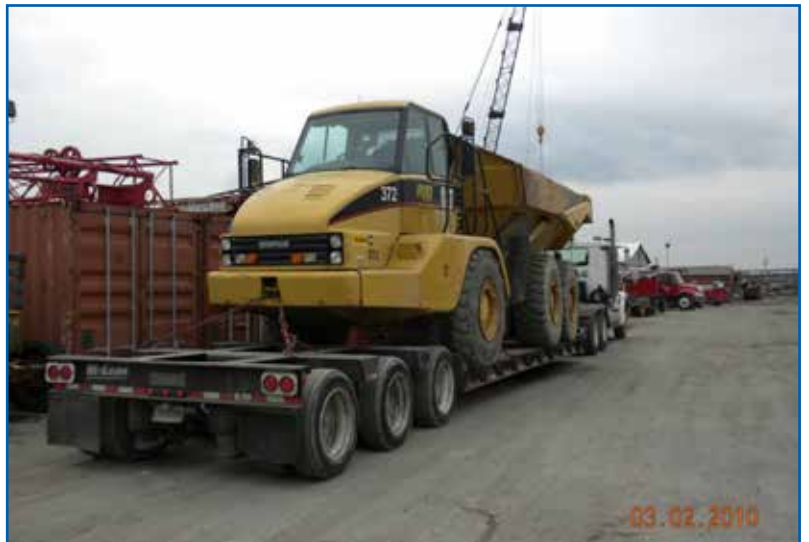
This truck, here mounted on a flatbed, is the type that will be used to move sediments. Sediments will be moved from the barge into dump trucks using the crane-mounted clamshell bucket; then sediments will be placed on the upland dewatering pad to drain water from sediments.
