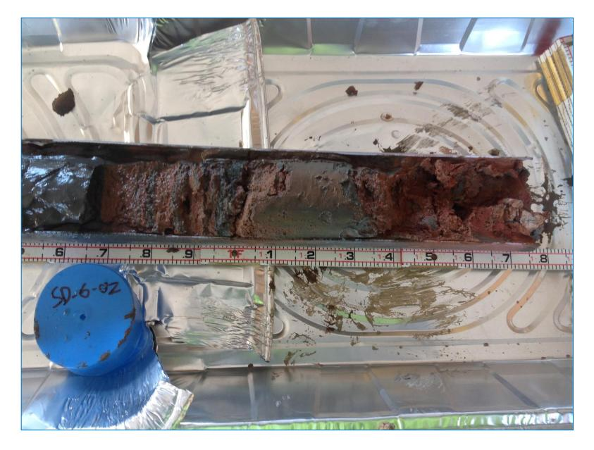
Samples were taken to confirm project goals were met. Clay indicates all sediments were removed at this location, since clay would have been the top layer when the cove was originally dredged in the 1940s before sediments began accumulating.
