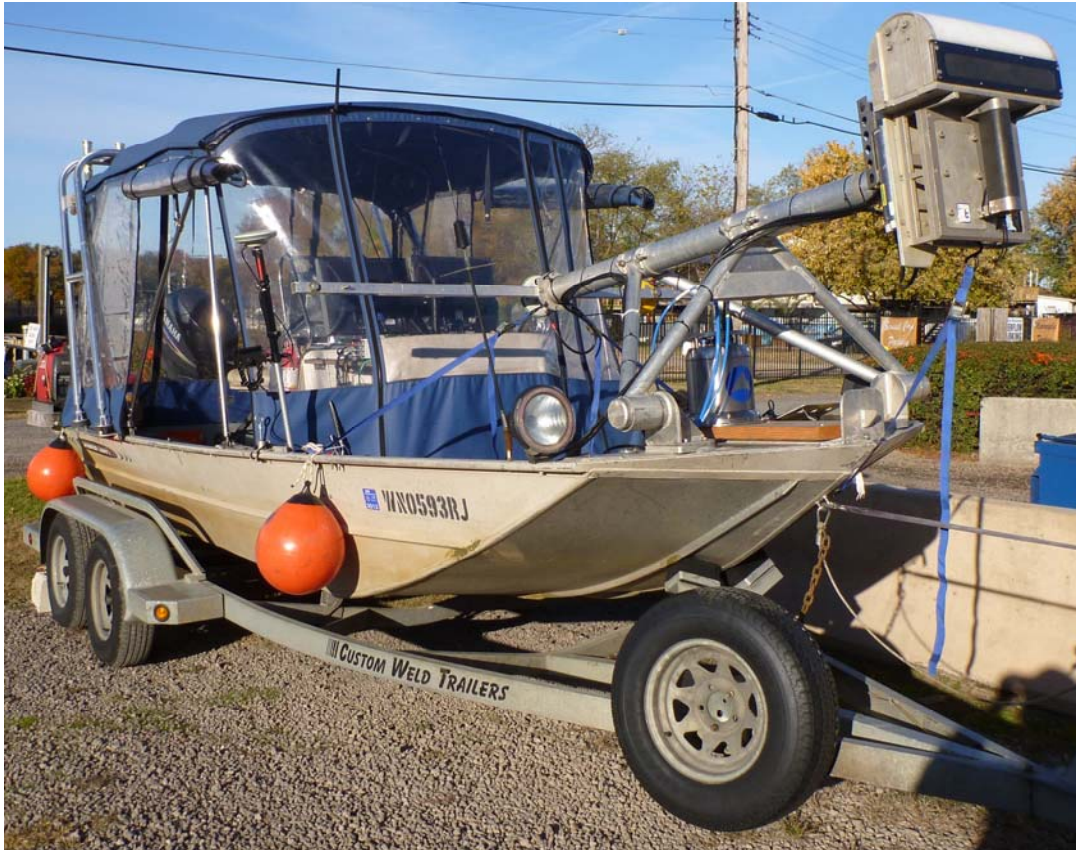
Figure 2-1. RESON SeaBat 7125 Multibeam Survey Vessel – R/V MIJITT
