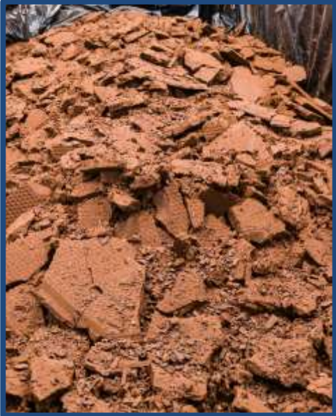
Filter cake in roll off awaiting disposal
