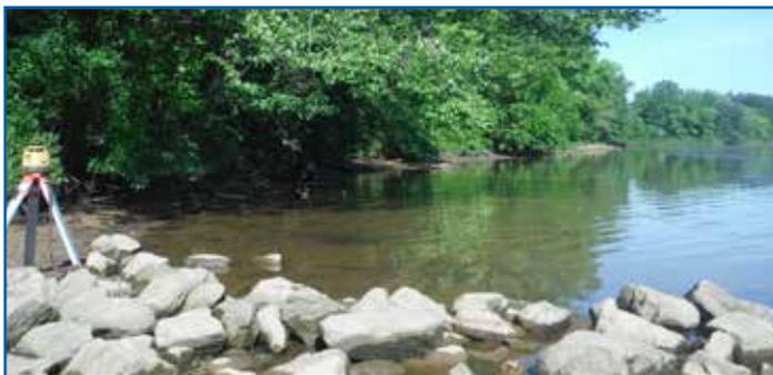
*To establish the elevation of the bottom of Cow Pen Creek, a laser level transmits a signal from a spot on the shore of the Creek to a receiving rod on the boat out in the creek, from which the depth from the laser to the bottom of the creek can be measured. By comparing this measurement with that from a spot with a known elevation, the elevation of the creek bottom is calculated.*
