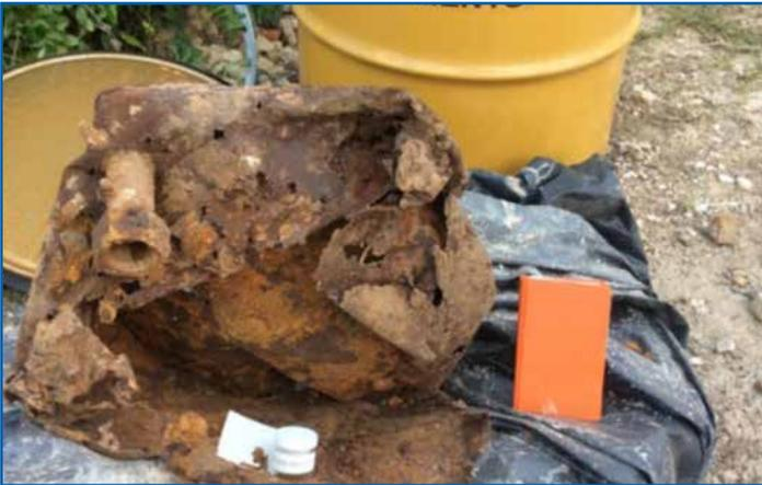
***The transformer housing found in Block G was sampled to determine whether polychlorinated biphenyls (PCBs) contamination were present, so it could be disposed properly.***
