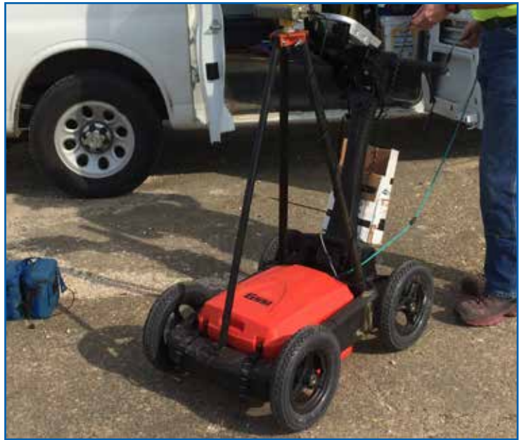
Ground penetrating radar unit used for geophysical surveying.
