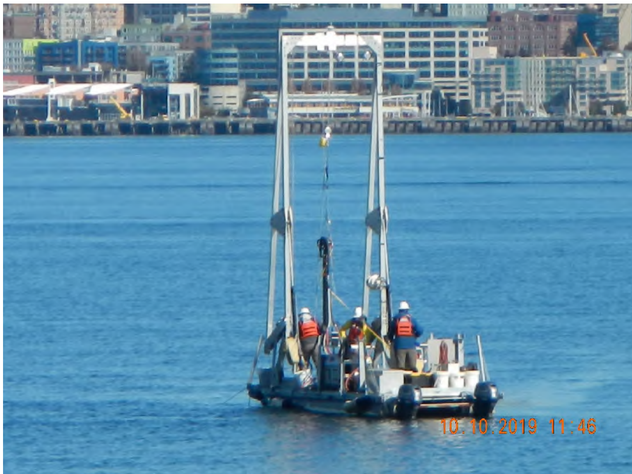
Photo 8 Sampling Vessel Collecting Core Sample
