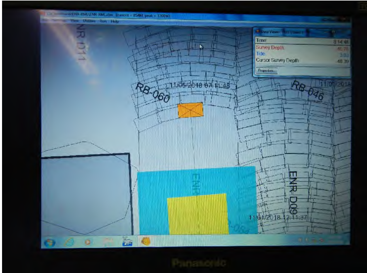
Photo 11 On-board Navigation System Bucket Swing Marks
