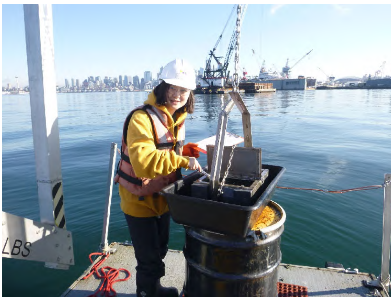
Photo 18 Collection of Sediment Samples after Placement of Enhanced Natural Recovery and Residual Management Layer Material
