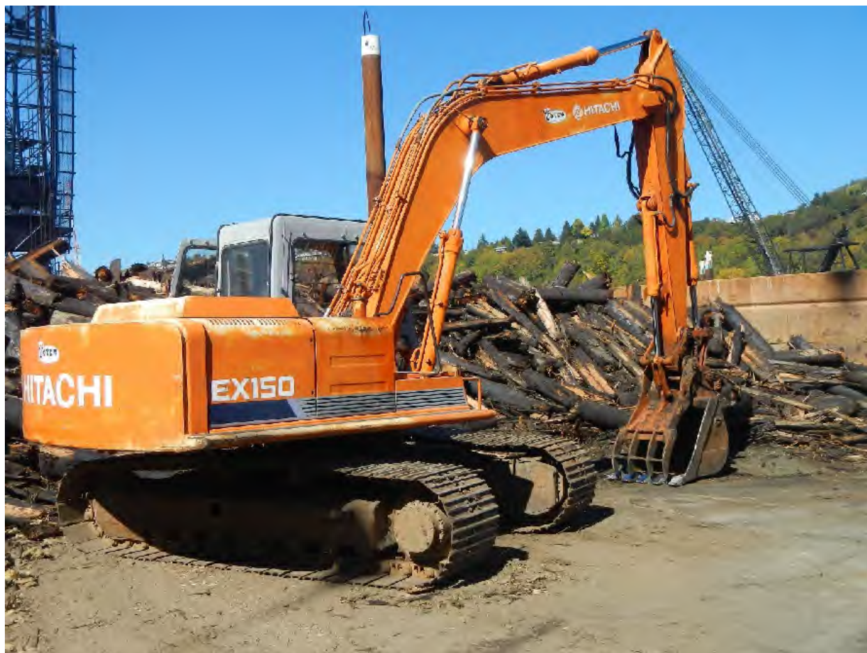
Photo 16 Excavator Used to Place Pilings in Containers
