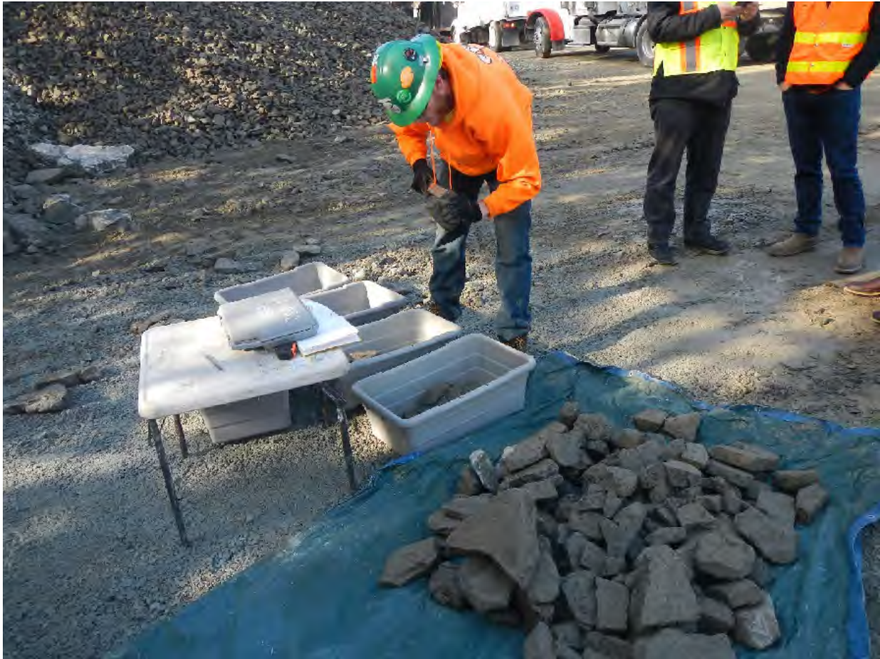
Photo 2 Backfill Material Being Measured to Determine if Material Meets Specifications
