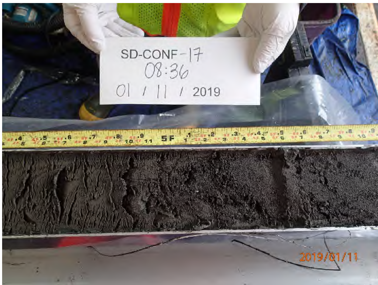
Photo 9 Core Sample that was Collected for Decision Unit Bottom Sampling
