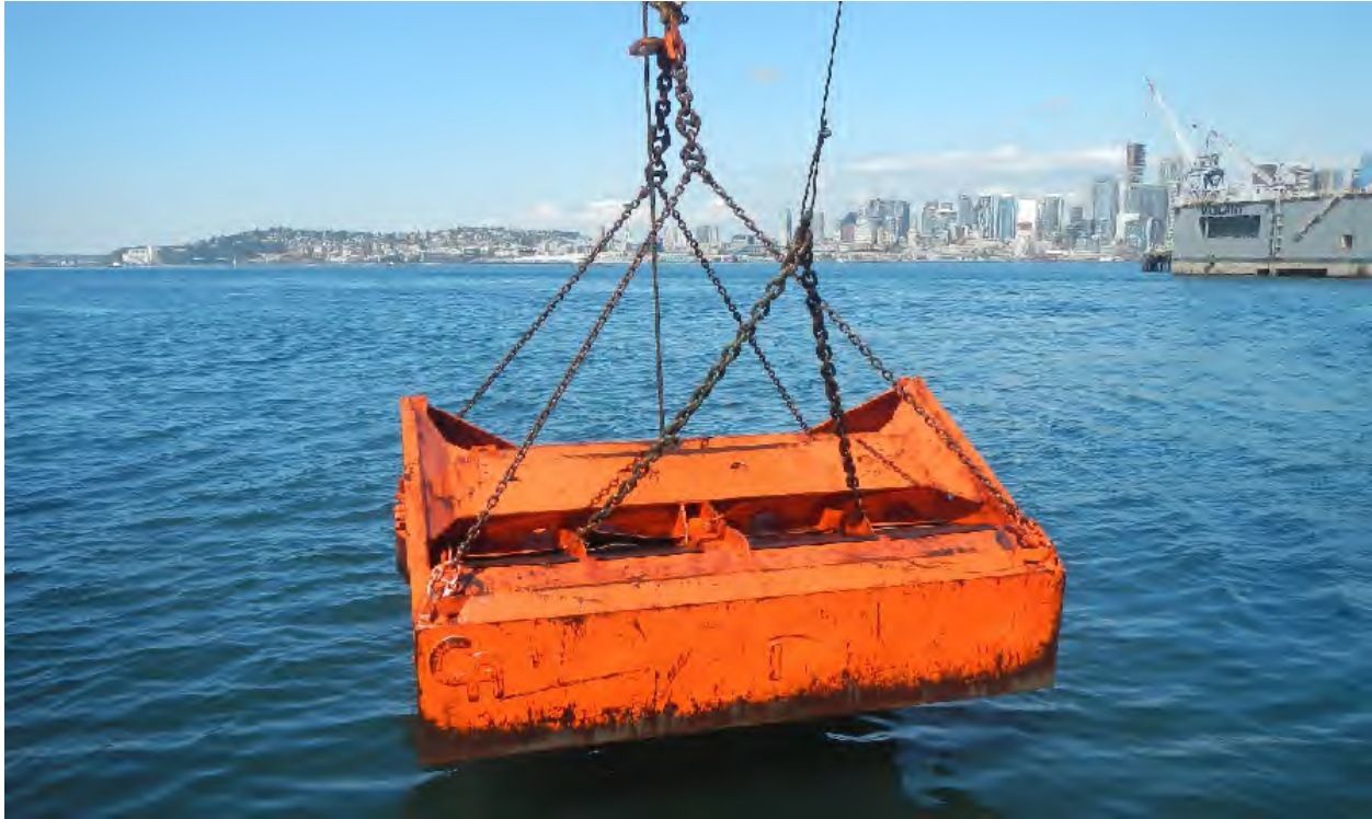
Photo 5 Environmental Dredge Bucket Used During Dredging
