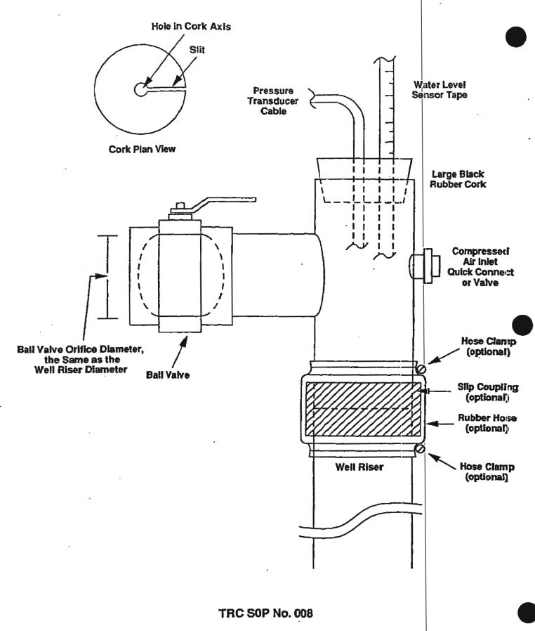
Pneumatic Slug Test Pressure Tree Assembly Schematic.
