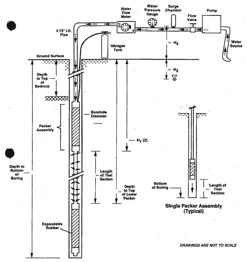
Double Packer Assembly and Associated Apparatus (Typical)
