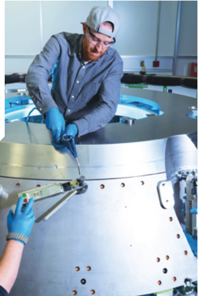
Employees assembling the forward bay cover for the Orion spacecraft.
