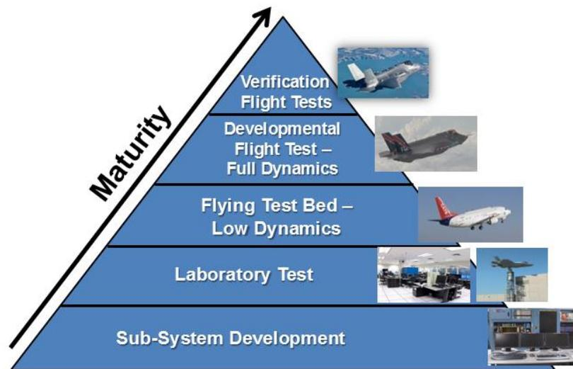
**Fig. 20 Test buildup methodology.**
