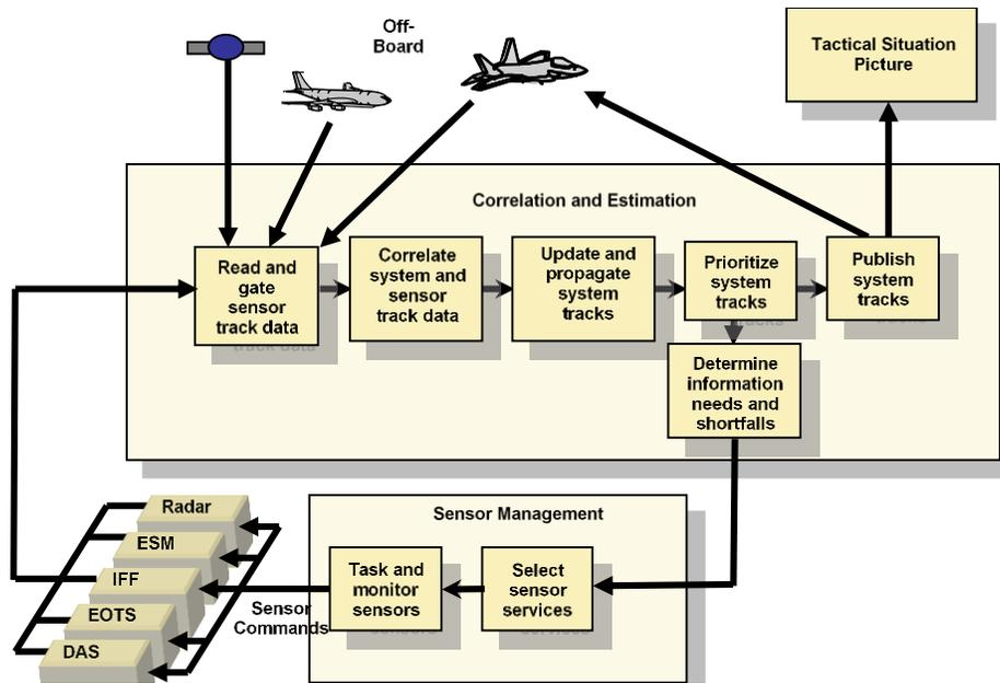
**Fig. 15 Closed-loop sensor data fusion.**
