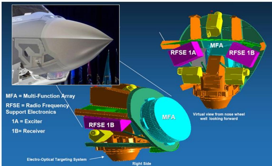
**Fig. 6 Installed radome and radar locations.**
