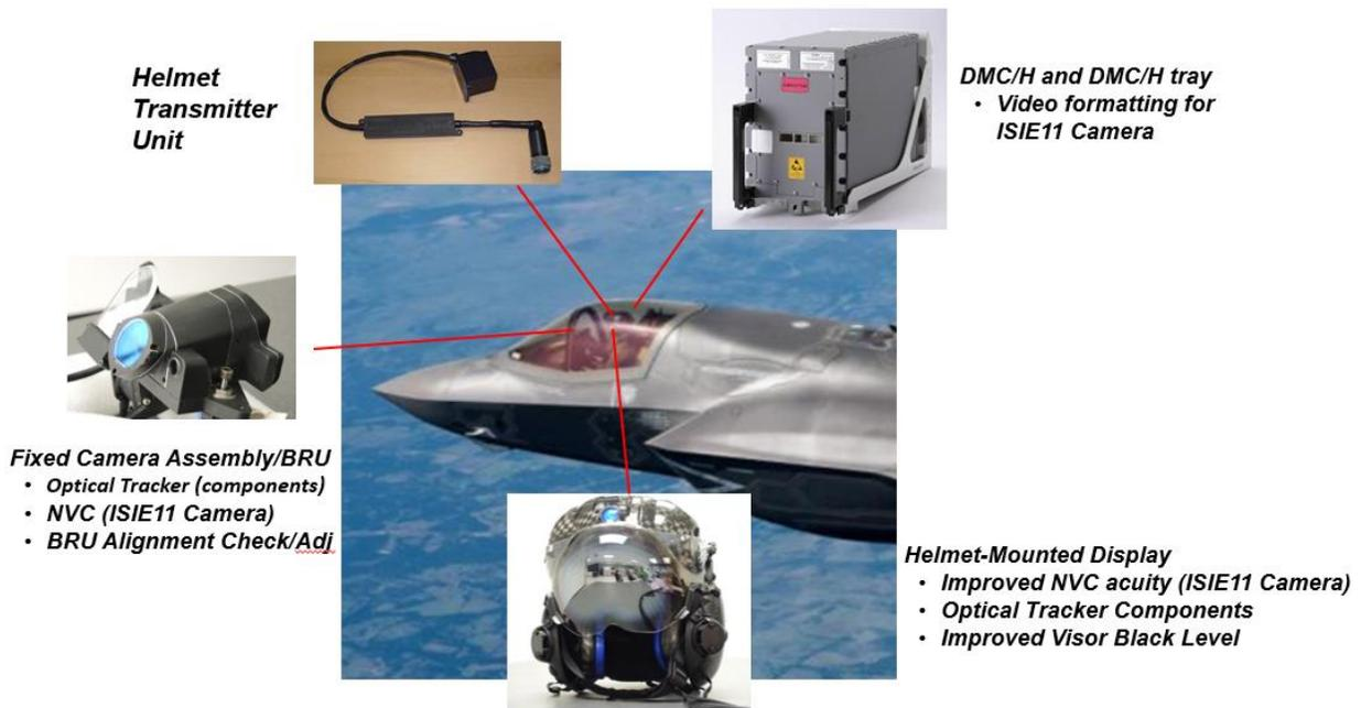
**Fig. 17 Gen III helmet-mounted display system.**
