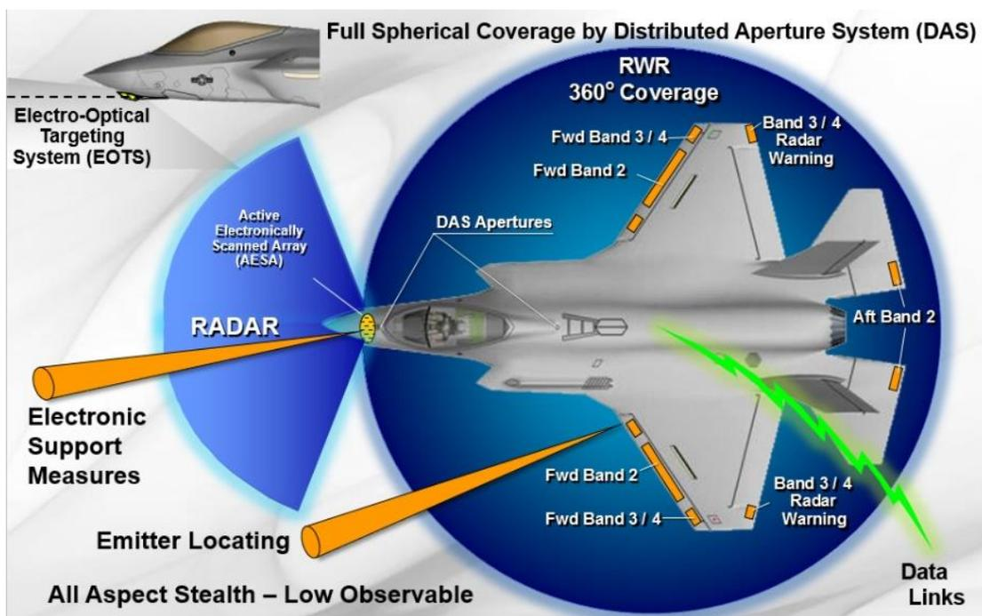
Fig. 4 F-35 installed sensor locations.
