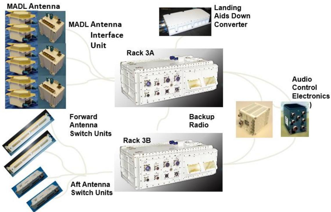
Fig. 14 CNI system components.
