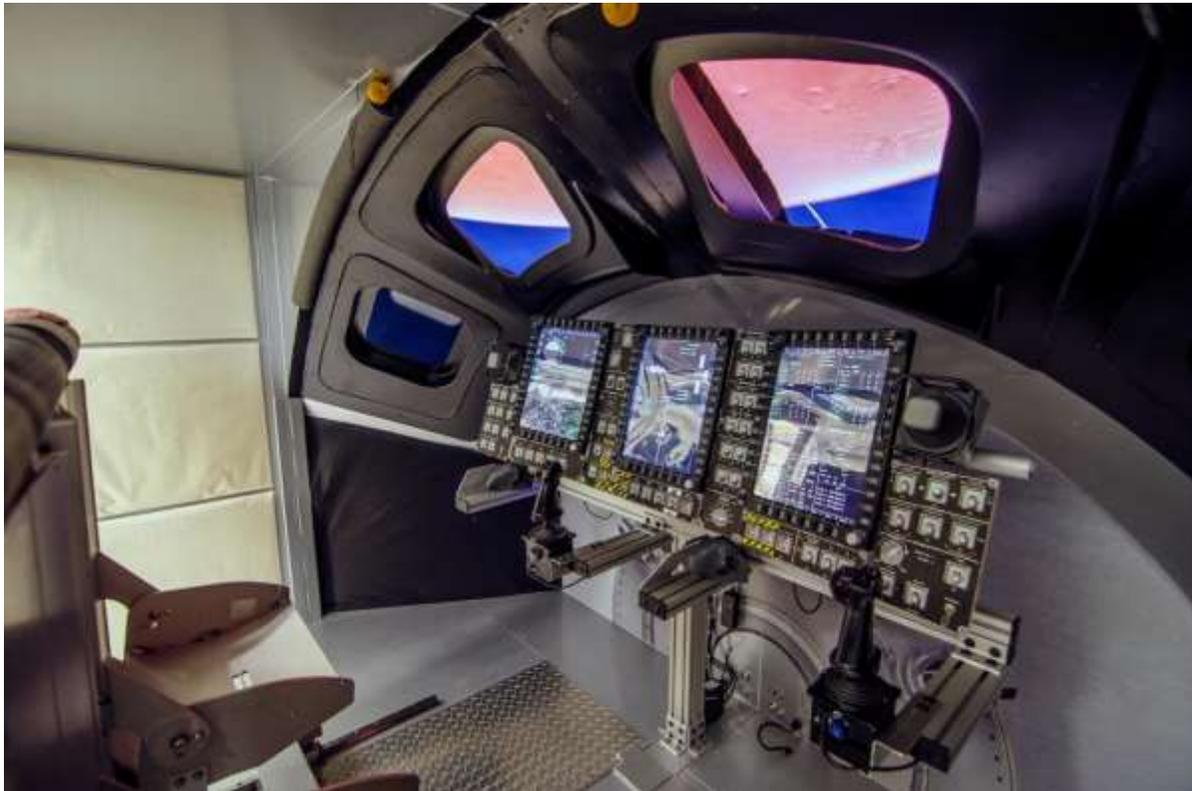
**Figure 6. Flexible Display Formats and electronic procedures enable extensive crew interaction with the Orion spacecraft.**
