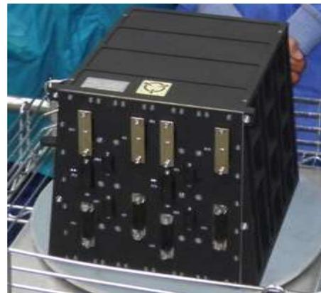
**Figure 4. Orion Vehicle Management Computer houses the Flight Control Modules that are the command source for the spacecraft and could minimize computing needed on the DSG.**
