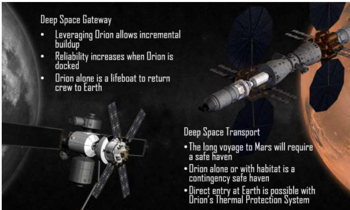
**Figure 8. Orion provides safe haven capability for the DSG and MBC.**
