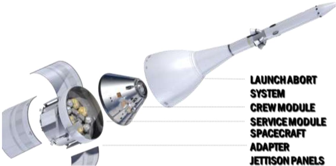
**Figure 2. The Orion Spacecraft Configuration**
