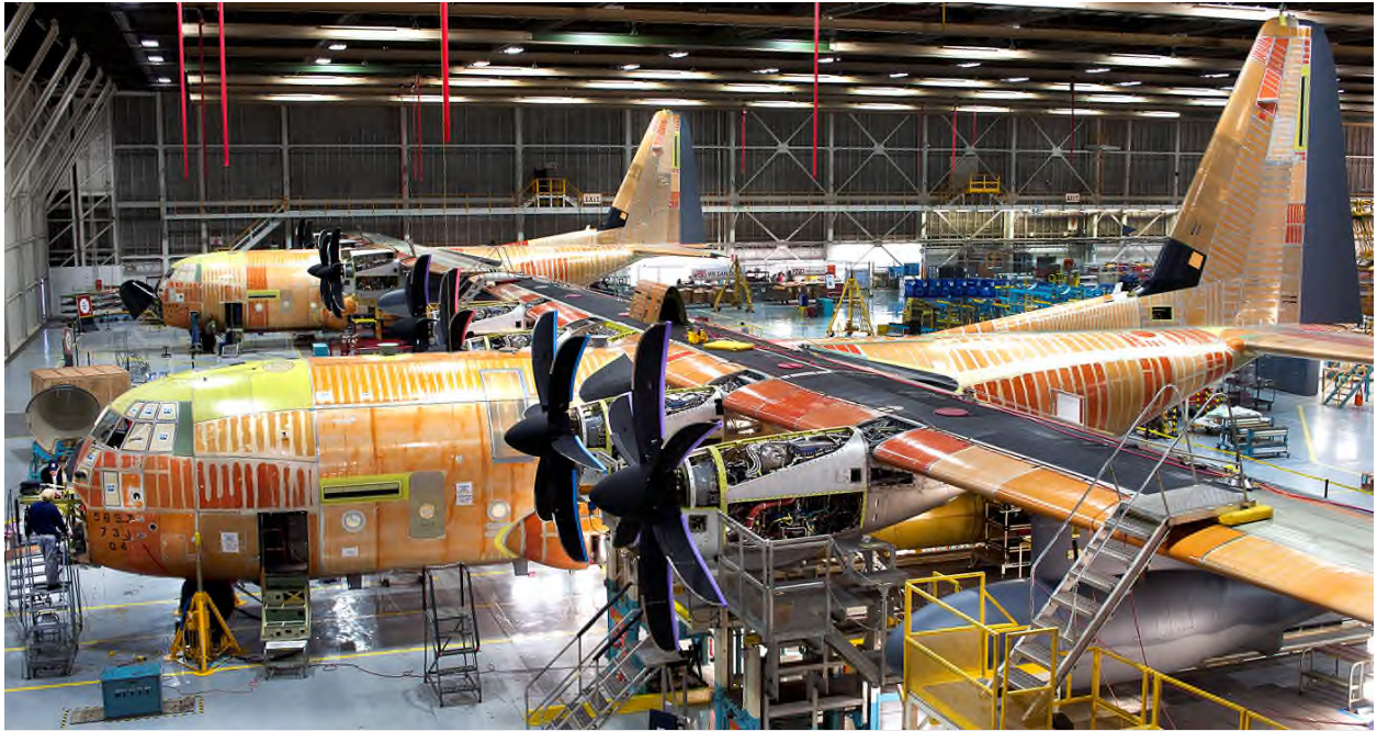
Two MC-130Js for U.S. Air Force Special Operations Command nearing completion on the C-130J production line at the Lockheed Martin facility in Marietta, Ga.
