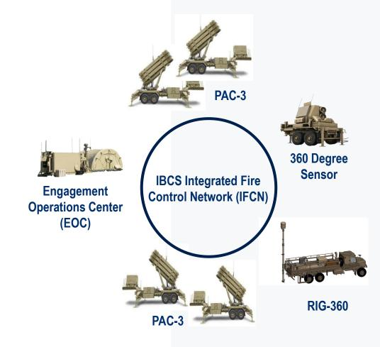
Networked enabled engagement capability using sensors on the IFCN
